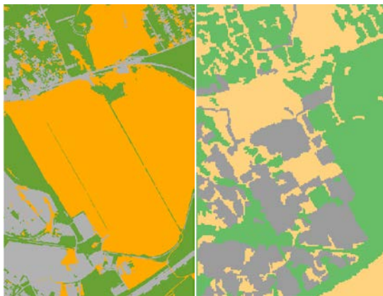
Fig. 11. The results of classification process in ArcGIS Pro (grey-built-up area, green-vegetation, orange-bare land)
