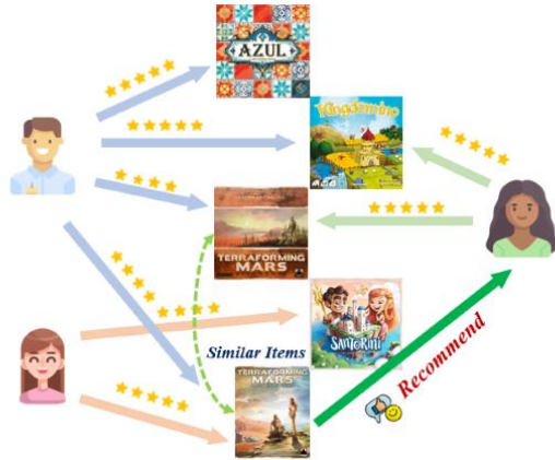
Fig. 3. Item-based collaborative filtering method example based on board game items. The recommendation based on similarity between rated games.
